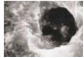
An example of hole detected by using our high voltage system = Pinhole 0.5µm photomicrograph
